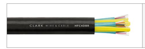
Four Channel Hybrid Fiber Cable For SMPTE 304/311 Format Cameras 16AWG conductors for extended distance runs Water Blocking Tape Barrier Direct Burial Construction CMR Listed for Permanent Install
