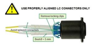
Avoid splayed connectors by using LCs without anti-snag collars and a boot diameter < 5 mm (available from suppliers as e.g. Corning).
