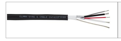
22AWG Signal Conductors 16AWG Auxiliary Conductors Overall Foil Shield with Drain Ideal for SMPTE Panels and Boxes Direct Burial Construction UL Riser Rated CMR
