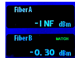
Example display of a broken fiber in the Fiber 1 position.
