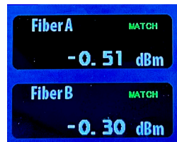
Example display when the cable under test is good.
