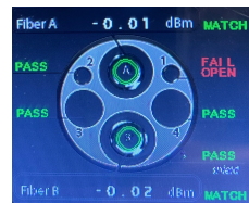
Example of display when there is an electrical open.
