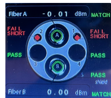
Example of display when there is an electrical short between conductors.
