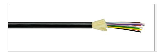
Heavy Duty Tactical Construction Single-Mode or Multi-Mode High Strength Coating and Buffer Overall Aramid Strength Member Polyurethane Jacket 2, 4, 6, 8 or 12 Fiber Elements
